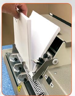
Book shaping spine formers enable the operator to insert diameters up to 50 mm. Coil diameters larger than 20 mm must use a 3:1 or 2.5:1 pitch large oval hole pattern.
